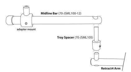
Note: When mounting the adapters or the midline bar use approxmately 10 in. lbs of torque to be assured the device is securely mounted.
